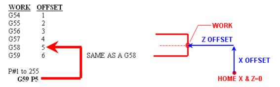
Another example of use would be making multiple turnings using the same code by providing an offset to do the other turnings. ie; G54 offset used for the first turning and then G55 Z ( offset amount ) such that the cutter would start at a different point along the Z axis for the next turning.
