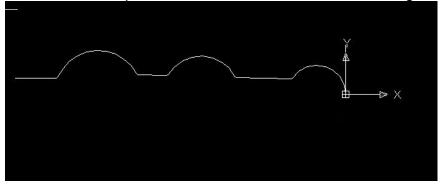
In order to cut the profile from beginning to end along the profile for the above piece the user must use a "point tool" and ground in such a fashion such that it will not gouge.
