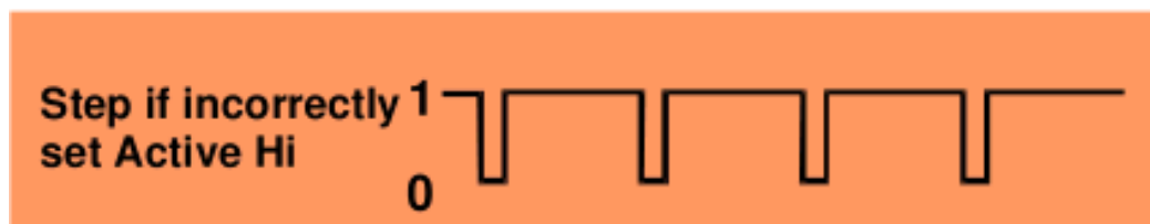
Figure 4.5 - Wrongly configured output alters step waveform
