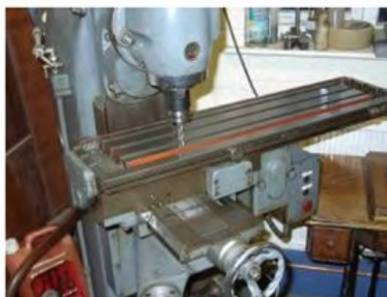
Figure 4.10 – Mill with tool at X=0, Y=0 position (note the dog is on limit switch)
