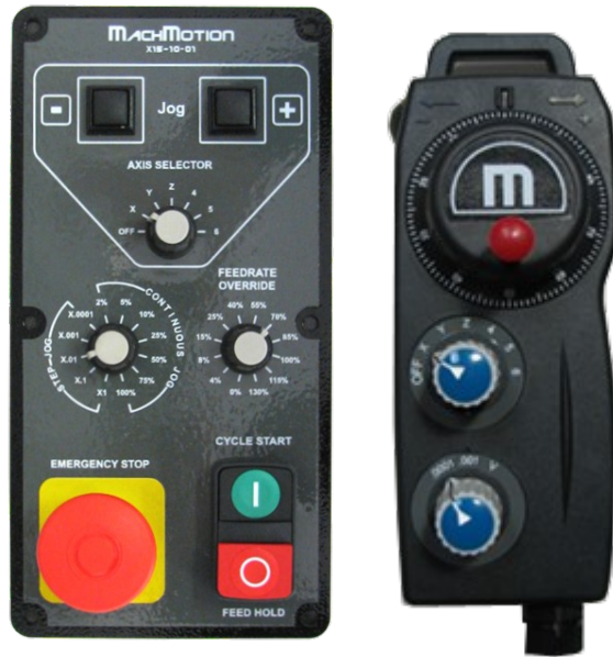
Figure 3-6: Control panel and pendant examples
